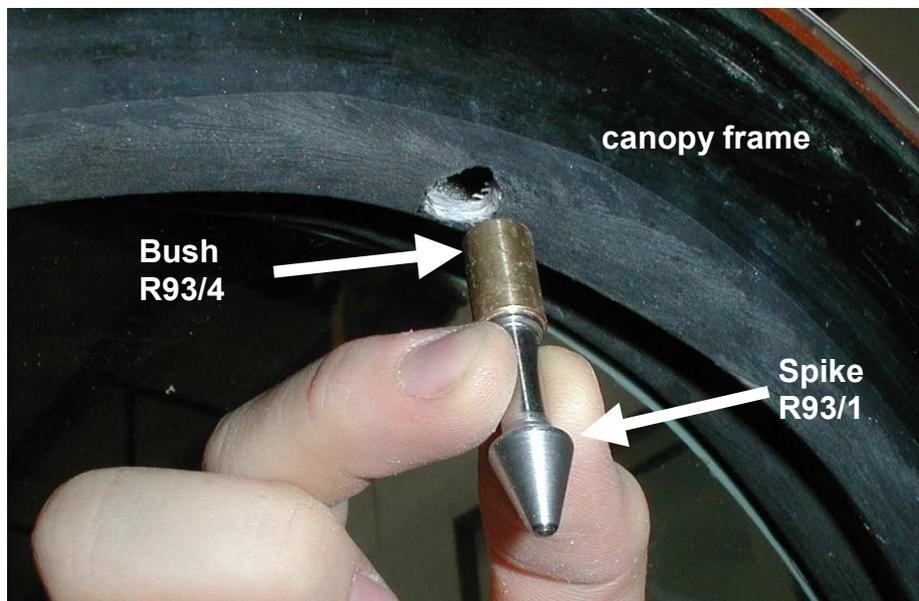
**Fig. 7: Hole in the canopy frame**
