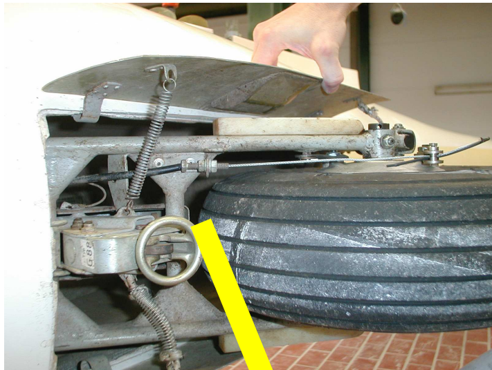
Figure 2: Overview showing the laying of the brake cable
